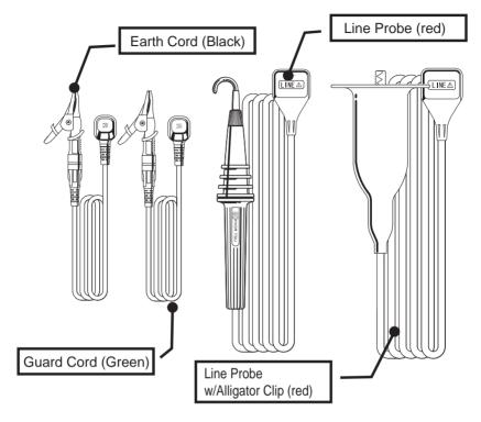
Depending on usage, either Line Probe or Line Probe with Alligator Clip is connected to the Line terminal.
