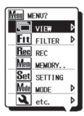
Move the cursor with the **UP/DOWN Keys** or **Shuttle Switch**, and confirm the selection with the **ENTER Key**. Pressing the **ESC Key** while the Menu is being displayed closes the Menu Window. Items displayed with "p" mark are accompanied with submenus. Press the **ENTER Key** to access to the submenus.
