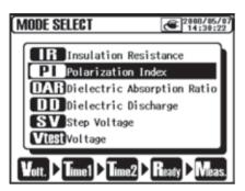
Move the cursor with the **UP/ DOWN Key** or **Shuttle Switch**, and confirm the mode with the **ENTER Key**.
